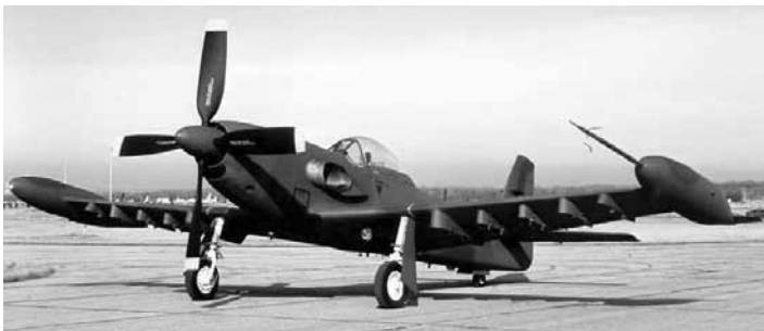
Figure 3-1. PA-48 Enforcer with weapon pylons and boom installed
