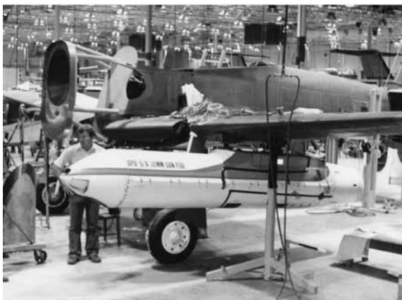
Figure 3-2. 30 mm Gun Pod Installation
