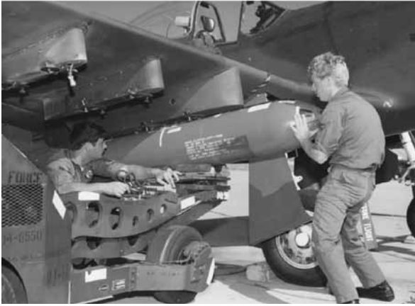
Figure 5-1. Loading a MK-20
